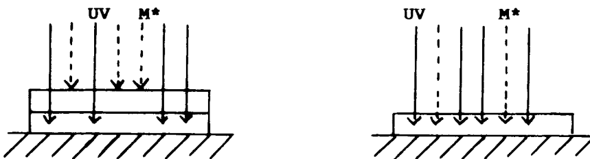
Fig. 2. Diagram of the experimentation on the direct energy transfer induced polymerization.
